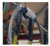
Disengage one of the hotsticks from one sleeve and use it pull the front of the cover down until it covers the insulator neck and hooks under the crown and/or tie wire. It is important to ensure the angle of the cover matches the angle of the insulator. Take your time.
