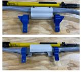
With points of each tool facing away from the cap, insert a tool into each sleeve. Tool handles will be facing as shown. It is necessary to have each handle on the lineman-facing side of the conductor during installation.
