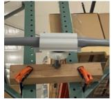
Once installed, the cap is locked into place and the sleeves are wrapped along the conductor.
