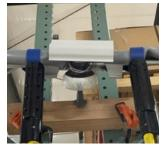
Using the tools to support the sleeves and guide the cap, snap the cap over the insulator pin.
