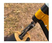
Tighten the clip with adjustable pliers.
